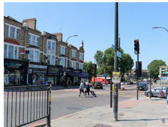
Many pedestrians cross New Cross Road across the desire line towards the bus stop on the other side of the station which more than 50m distance from the only one, therefore there is opportunity for additional crossings.
